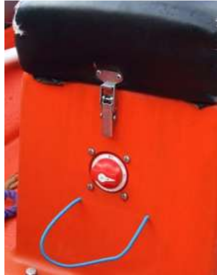
Isolator switch ON
